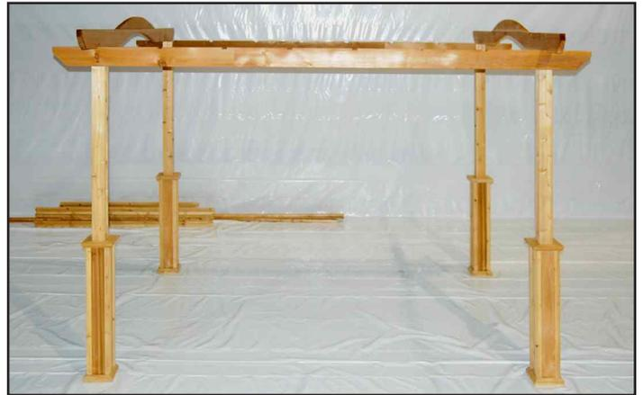
8. Place pergola assembly in it's final location. A level and sturdy foundation is required. Measure the distance between the legs to ensure they are the same. Match measurements of line to line, dashed to dashed, dots to dots. Adjust, if necessary. See diagram.
